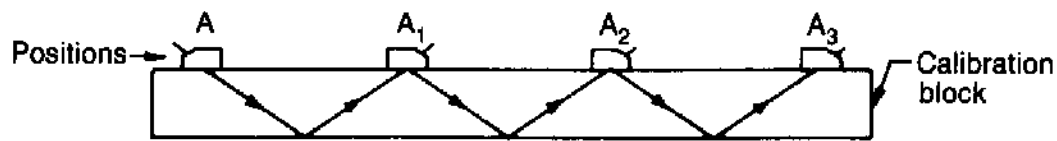
(a) Probe position on calibration block
